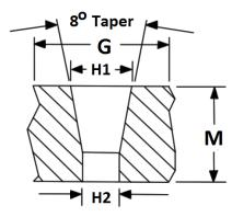
When installing inserts into a boss, the minimum diameter "G" of the boss should be at least 1.5 times the diameter of the insert.
